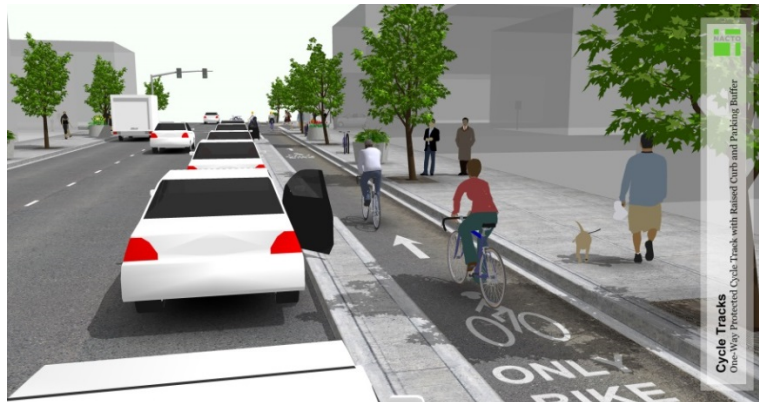
(Protected bike lane)
